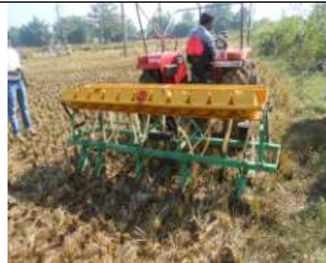
FLD on Zero till seed cum fertilizer drill for sowing wheat
