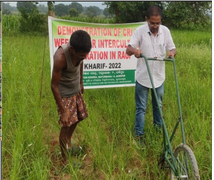
FLD on Demonstration of CRIJAF weeder for intercultural operation in ragi
