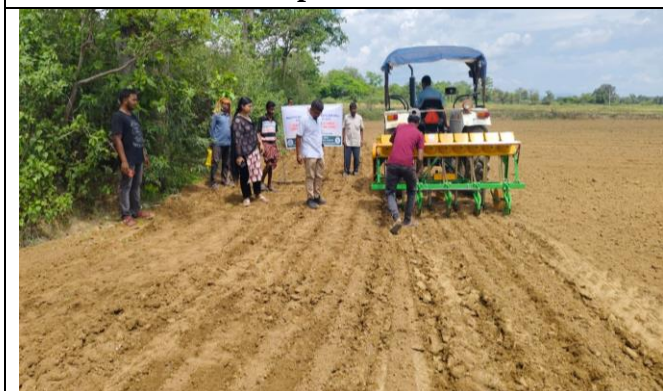
Demonstration on Tractor drawn seed cum fertilizer drill for direct seeding of rice
