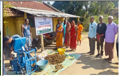
Demonstration of 0.5 hp motor operated mini ragi thresher cum pearler
